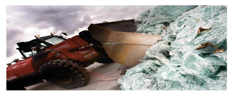
Saint-Gobain Building Glass innovative use of cullet in the glass manufacturing process has always been a key differentiator for the business. Saint-Gobain Building Glass currently operates the UK's largest cullet return scheme and since the introduction of cullet use in the manufacture of float glass, we have been able to increase the amount of recycled glass utilised to 35% - rising to 41% in some cases.
